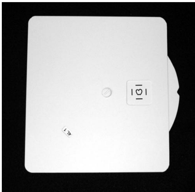
FIGURE 1. Crowded Single Symbols Visual Acuity Test. A single symbol surrounded by four crowding bars at 0.5 optotype width is presented in a window in the mask covering the disk. A second, small window indicates the specific test age (4 years) and eye (left) being tested, and the place in the sequence of four optotypes (no. 1) of the symbol that is shown in the window. Four disks were used: one for each eye in 3-year-old children, each containing four 5/16 and four 5/12.5 optotypes, and one for each eye in 4- and 5-year-old children, each containing four 5/12.5 and four 5/10 optotypes. Test distance was 5 ft.
